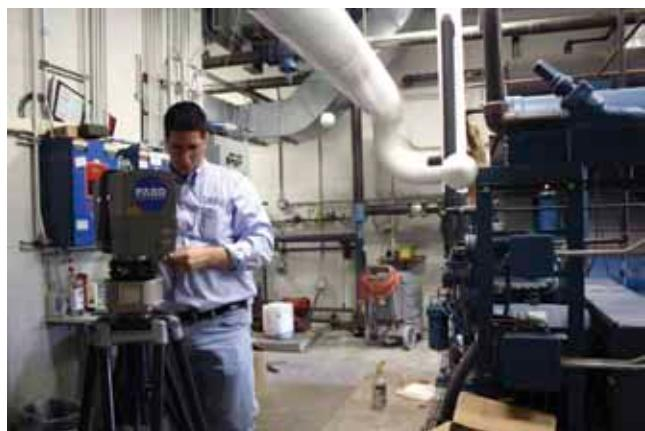
Through a previous customer referral, GKS Global Services was chosen as the 3D scanning provider by the engineering company. GKS was brought in to perform a scan of the entire mechanical room to create a precise 3D model to facilitate the equipment install.
