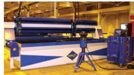
The investment in tools like the FARO Laser Tracker has made WARDJet more efficient in production by gathering infinitely more data in a shorter period of time. The ultimate result has been a higher accuracy waterjet cutting machine with improved reliability.
