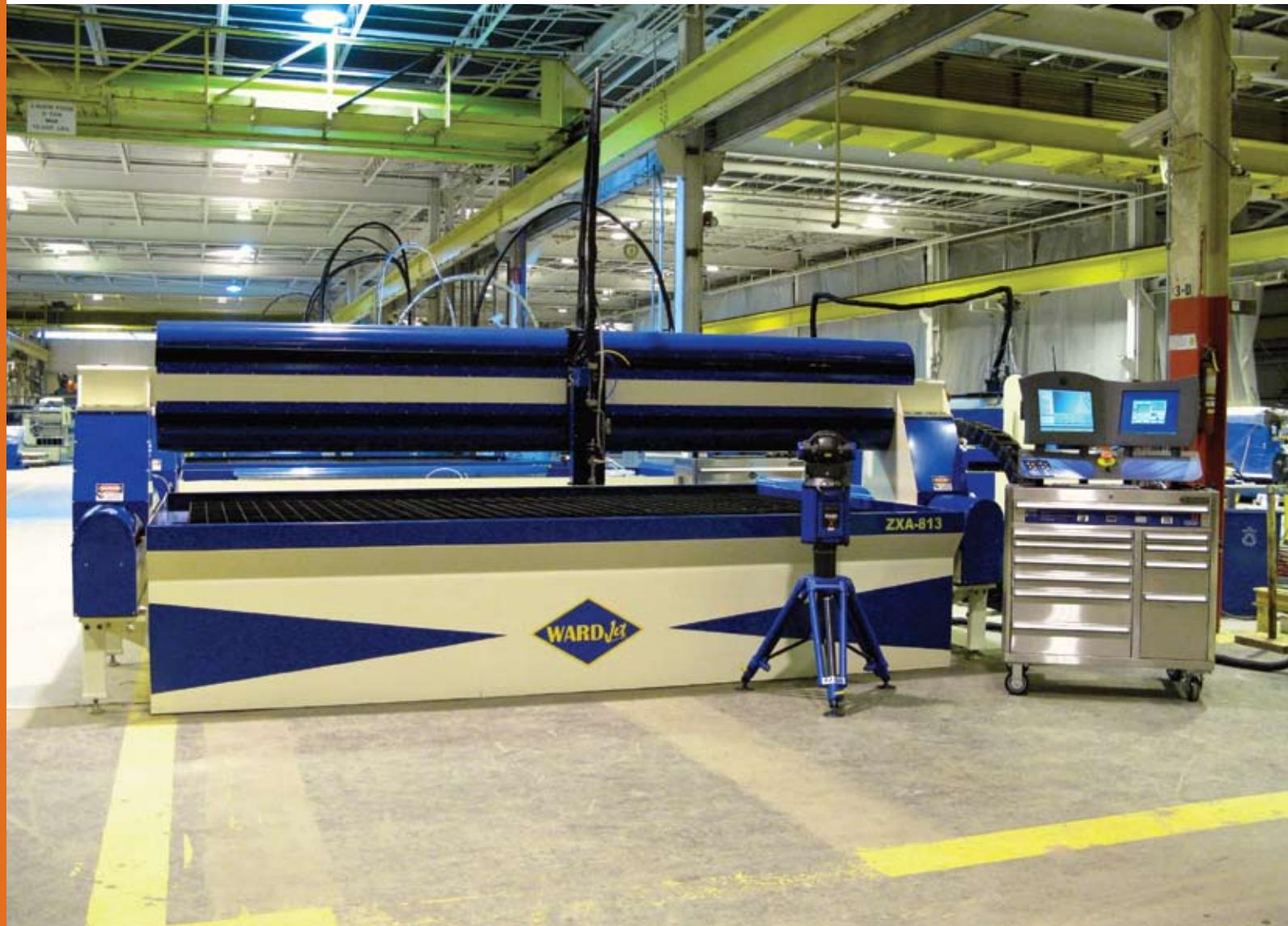
Using previous methods, laser calibration of WARDJet's waterjet machines would take up to three hours. With the FARO Laser Tracker, they can now do the same work in close to one hour. The FARO Laser Tracker has also allowed them to verify and analyze parts of their machines that they previously couldn't, taking their calibration, quality, and R&D to a whole new level.
